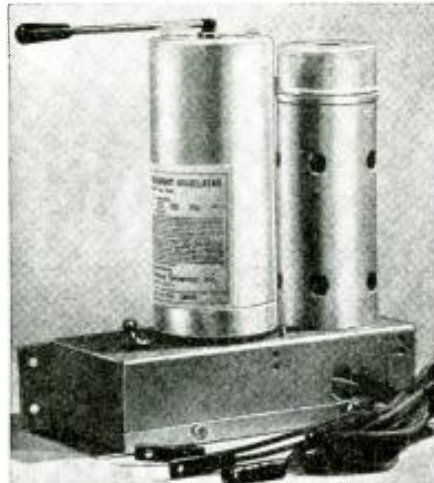
New Beat Frequency Oscillator (No. 325)
